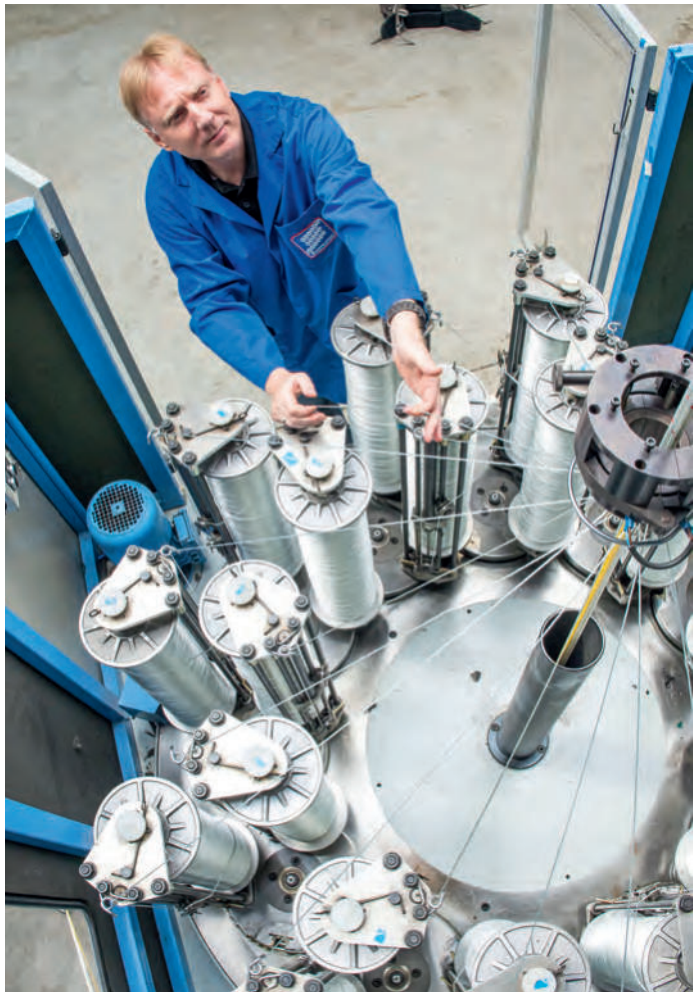
Final inspection of the tensioned yarn before production begins.
