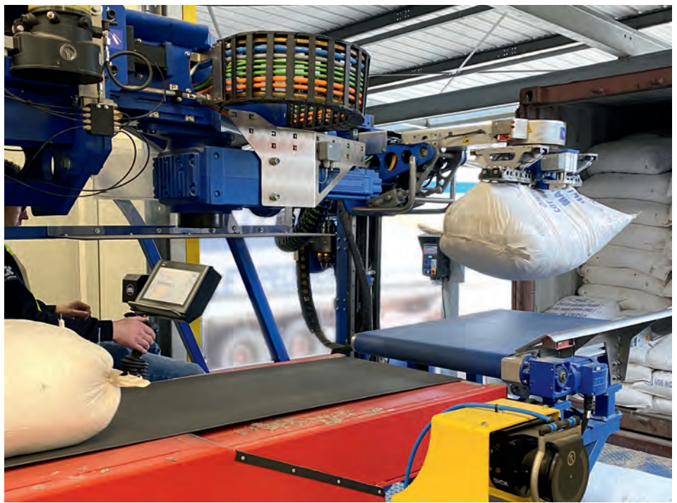
At Hofmann Group, a robot takes over the unloading of heavy bagged goods. This relieves the employees, as they only need to monitor the process.
