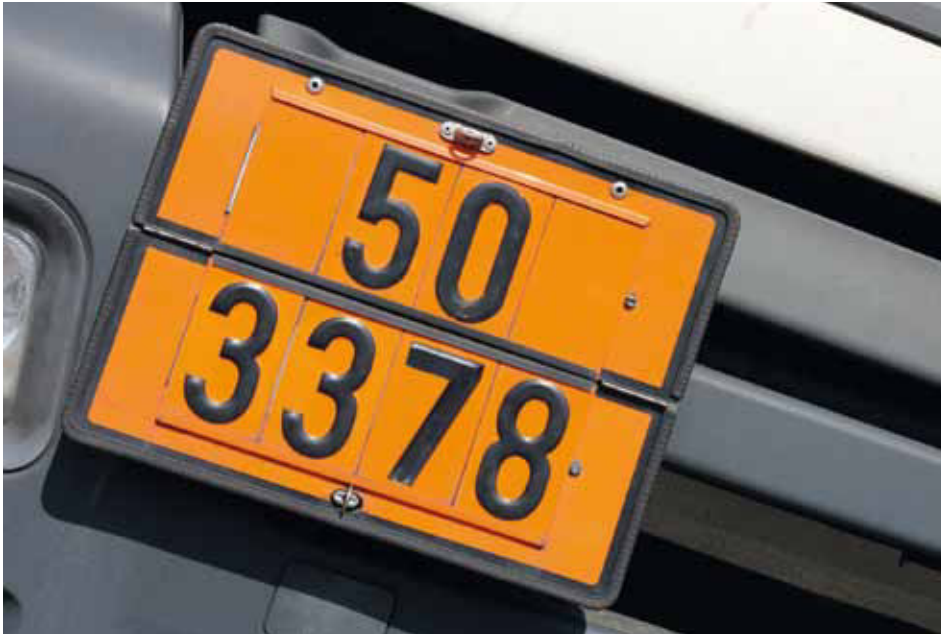
Thanks to the orange signs that classify the shipment (here sodium carbonate peroxohydrate with UN no. 3378 and hazard no. 50) and whose use is mandatory on lorries transporting hazardous materials, paramedics and firefighters know exactly how to handle the shipment in case of an emergency.
