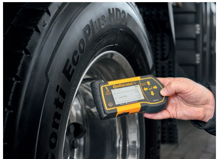
The ContiPressureCheck™ hand-held unit is used to measure the tyre pressure.
