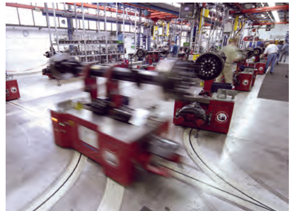
Final assembly of the axles occurs flexibly in three production lines in Bessenbach.
