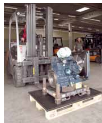
Non-slip mats prevent shipments from moving where they are not supposed to.
